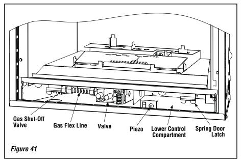
Refer to *Figure 42* and insert the last length of gas pipe with its attached shut-off valve into the lower control compartment, and pass it through the gas line access hole on the left side of the appliance outer wrapper.
